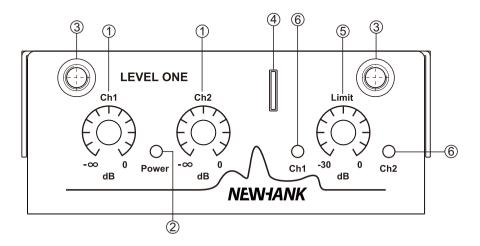
The front panel of the Level One contains all the controls and indicators and mechanical parts to lock the housing
